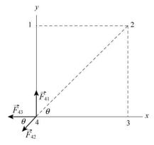
$$F_4 = F_{4x}^2 + F_{4y}^2 = \left[ \left( -\frac{3\mu_0 i^2}{4\pi a} \right)^2 + \left( \frac{\mu_0 i^2}{4\pi a} \right)^2 \right]^{1/2} = \frac{\sqrt{10}\mu_0 i^2}{4\pi a} = \frac{\sqrt{10} 4\pi \times 10^{-7} \text{ T} \cdot \text{m/A}}{4\pi 0.135 \text{m}} = 1.32 \times 10^{-4} \text{ N/m}$$
