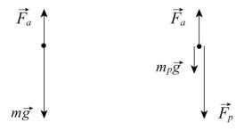
$\vec{F}_a$  is the force of the air on the parachute and  $m\vec{g}$  is the force of gravity. Application of Newton's second law produces  $mg - F_a = ma$ , where a is the acceleration. Solving for  $F_a$  we find
