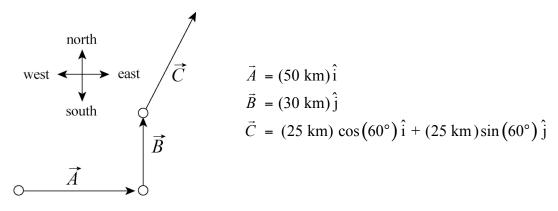
(a) The total displacement of the car from its initial position is represented by
