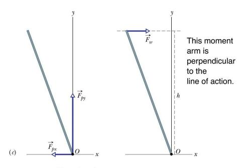
Choosing the rotation axis here eliminates the torques due to these forces.
