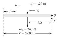
Requiring that  $\Sigma \tau = 0$  about an axis through point O and perpendicular to the page gives
